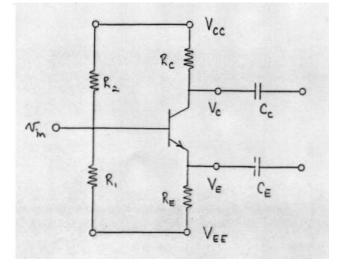
Before you come to lab, you should complete the homework problems (problems 8.7 and 8.8 in Sprott) that involve designing and calculating the properties of a common emitter amplifier.
