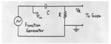
[Note that  $v_R(t)$  is proportional to I(t)] as a function of frequency. Assume that the frequencies you read from the dial of the function generator are correct. Take measurements for something like 15 points from f = 50 Hz to f = 15 kHz, increasing f by roughly a factor of 1.5 at each step. Make sure it is clear in your notebook how the various quantities in the table were determined. Use the DMM to measure the two voltages (the DMM reads the RMS voltage).
