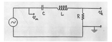
(a) Measure  $|v_{in}|$ ,  $|v_R|$  and  $\Phi$  for frequencies from 200 Hz to 25 kHz. You will need to take quite a few points near the resonant frequency, so that you can map out the shape of the resonance curves.
