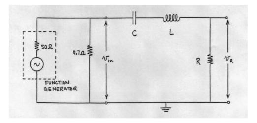
Depending on the apparatus available, use one of the two configurations given in the table below The circuits have  $Q \approx 10$  at the fundamental frequency, and a resonance width of a few hundred Hz. Note that on the capacitance decade boxes, MF means  $10^{-6}$  F. Set the function generator for about 75% of maximum output, and trigger the scope on the output of the function generator. All measurements are to be made with the scope.
