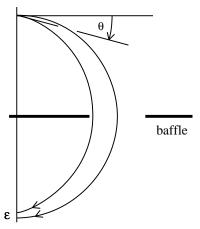
Because  $\sin^2\theta$  changes slowly near  $\theta=0,\,\epsilon$  is very small. A baffle with a slit is used to restrict the detected particles to those with  $\theta$  small. In this spectrometer the restriction is:
