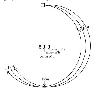
Note that the particles will pass through a focus point one diameter away from the source. Of course, if the angles are very large then the particle will pass near the focus. You may like to show that the particle will miss the focus by a distance  $\epsilon$ .
