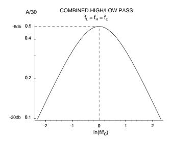
Therefore, the maximum gain of the stage is  $1/2(R_1/R_F) = 15$  at  $f_{\circ}$ , and drops off  $\propto f$  for  $f \ll f_{\circ}$  and as 1/f for  $f \gg f_{\circ}$  – both 6 *db per octave*. What is  $f_{\circ}$  for the given component values?
