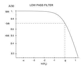
With **both** capacitors, the gain is just the **product** of these two curves. Since  $f_1 = f_2 \equiv f_{\circ}$ , the result is :
