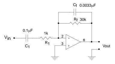
Ignoring the capacitors for a moment, this is just an inverting amplifier with a gain of  $R_F/R_1 = 30$ . The addition of  $C_1$  introduces a high-pass corner at  $f_1 = 1/2\pi R_1 C_1$  that reduces the gain at **low** frequencies, ie  $f \ll f_1$ :
